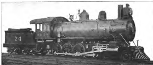
Fig. 73. Twelve-Wheel (4-8-0) Locomotive. Built by the Baldwin Locomotive Works for the Duluth & Iron Range. Cylinders 22 in. x 26 in., Diameter of Drivers 54 in., Weight on Drivers 140,060 lbs., Total Weight 172,260 lbs.
